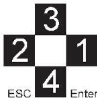
The two outer buttons are labeled „ESC“ and „ENTER“; they function much in the same manner as their counterparts on a computer keyboard. The two inner buttons serve as up- and down-arrow keys; they are the Scroll buttons used for stepping up and down through the menu lists and items viewed in the display. The QUATRIX's display shows one menu item at a time.
